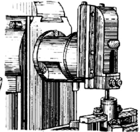
Fig. Slotting attachment
