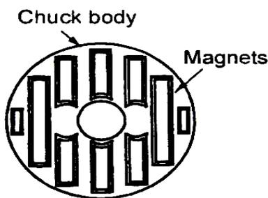
Fig. Magnetic chuck
