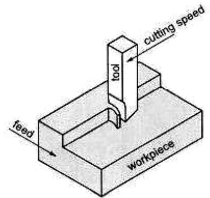
**Fig. 3 (b) Principle of producing flat surface**
