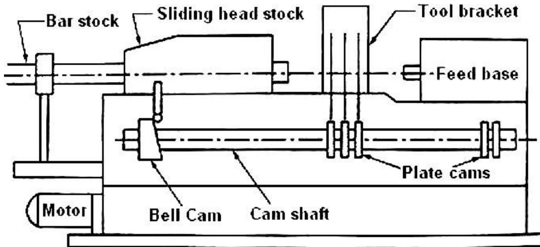
**Fig. Swiss type automatic screw machine**
