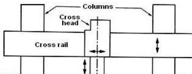
Fig. Multiple head type horizontal boring machine
