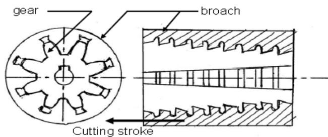
Machining external gear teeth by broaching.
