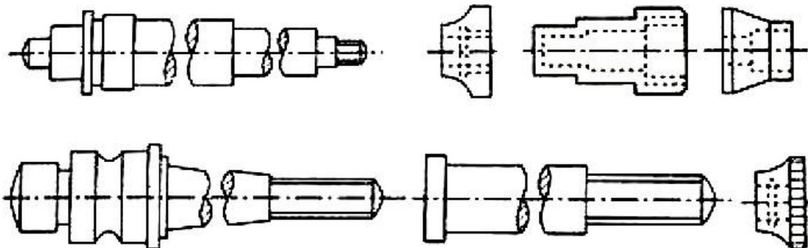
**Fig. Parts produced on multi spindle automatic lathe**
