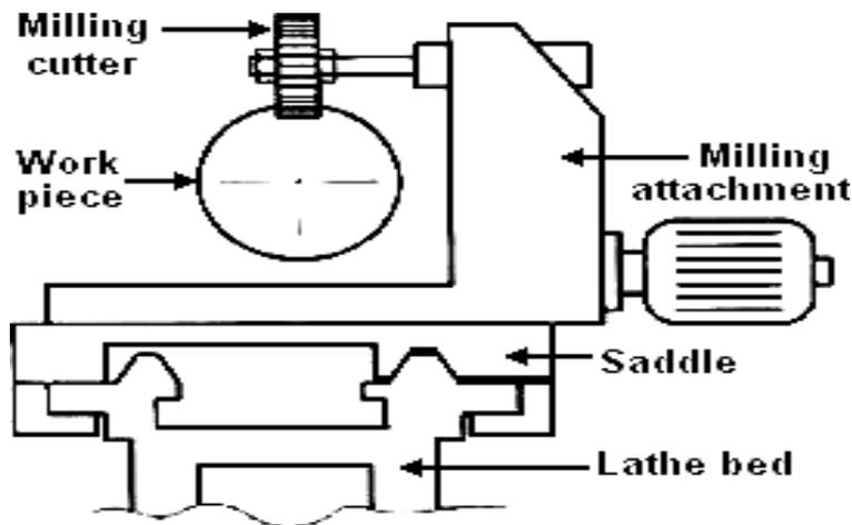
Fig. (b) Milling attachment
