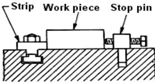
Fig. 18 Use of strip and stop pin
