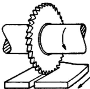
Fig. Parting by slitting saw
