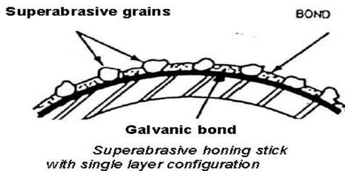
With the advent of precision brazing technique, efforts can be made to manufacture honing stick with single layer configuration with a brazed metal bond. Like brazed grinding wheel such single layer brazed honing stick are expected to provide controlled grit density, larger grit protrusion leading to higher material removal rate and longer life compared to what can be obtained with a galvanically bonded counterpart.
