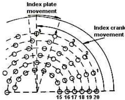
Fig. An example of compound indexing
