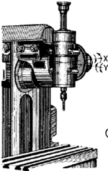
Fig. Universal milling attachment
