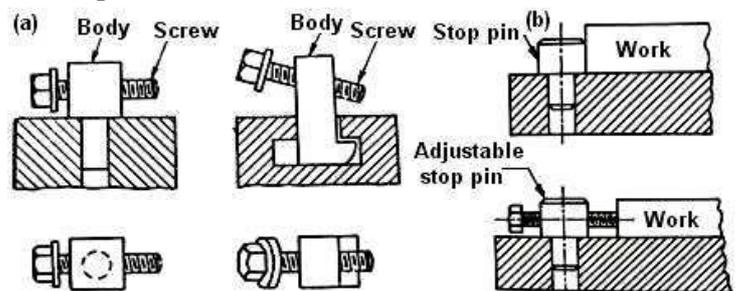
Fig. (a) Stop pins and (b) Use of stop pins
