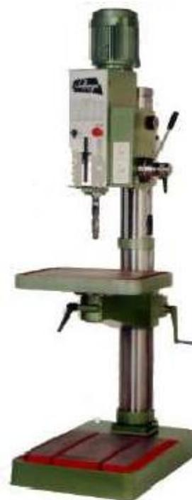
**Fig. Pillar drilling machine**
