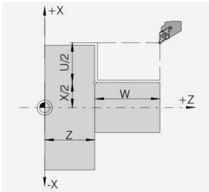
G20 Turning Cycle – CNC Lathe Fanuc 21 TB
