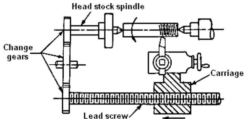
**Fig. Principles of thread cutting**
