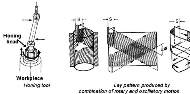
The honing stones are given a complex motion so as to prevent every single grit from repeating its path over the work surface. The critical process parameters are:
