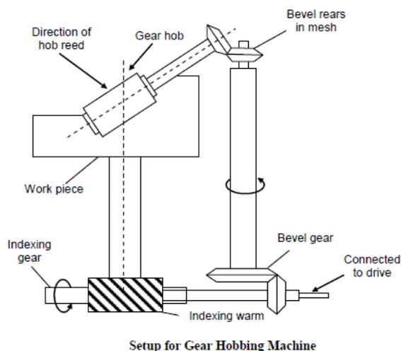
In this process the gear hob is fed against the gear blank along the face of the blank and parallel to its axis. This is used to make spur and helical gears.
