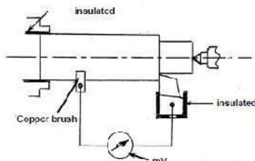
Fig. Tool-work thermocouple technique of measuring cutting temperature.
