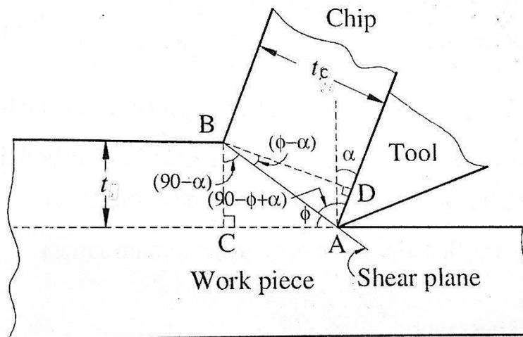
Shear angle  $\alpha$  is defined as the angle made by the shear plane with the direction of the tool travel if
