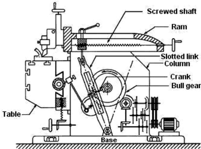
**Fig. 3 (a) Kinematic system of a shaper**
