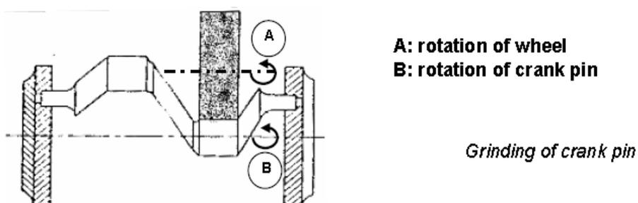
Cam and camshaft grinders are essentially subsets of cylindrical grinding machine dedicated to finish various profiles on disc cams and cam shafts. The desired contour on the workpiece is generated by varying the distance between wheel and workpiece axes.
