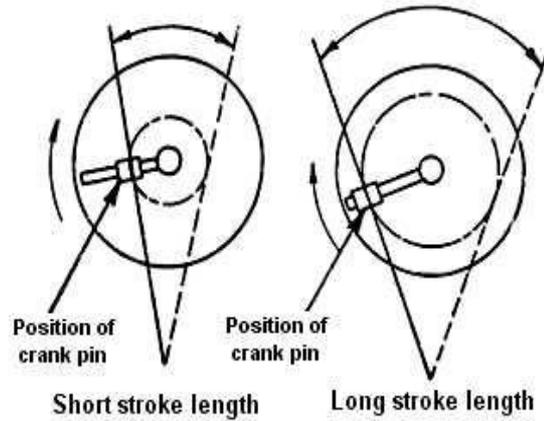
**Fig. (a) Arrangement of bull gear sliding block**
