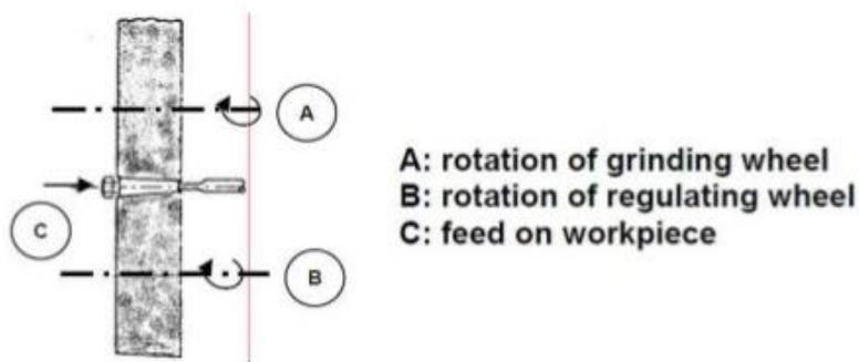
End feed grinding is used to produce taper, either the grinding wheel or regulating wheel or both are formed to a taper. The work is fed lengthwise between the wheels and is ground as it advances until it reaches the end stop.
