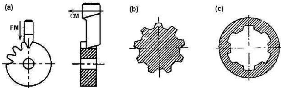
**Fig. Machining of (a) External gear (b) External splines and (c) Internal splines in a shaper**
