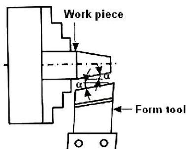
Fig. Taper turning by a form tool
