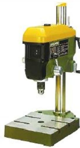
**Fig. Table top sensitive drilling machine**
