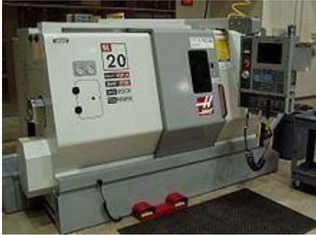
The first NC machines were built in the 1940s and 1950s, based on existing tools that were modified with motors that moved the controls to follow points fed into the system on punched tape. These early servomechanisms were rapidly augmented with analog and digital computers, creating the modern CNC machine tools that have revolutionized the machining processes.
