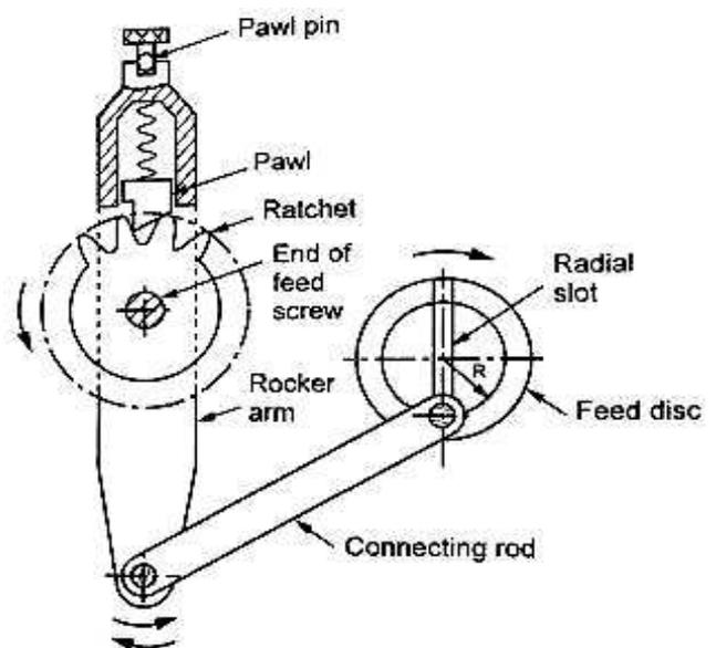
The feed mechanism in which the feed is given at the end of each return stroke is known as **feed mechanism**.
