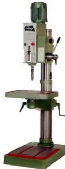
**Fig. Pillar drilling machine**
