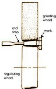
It is similar to plunge or form grinding, the regulating wheel is drawn back so that workpieces may be placed on the work rest blade. Then it is moved into feed the work against the grinding wheel. This method is useful to grind shoulders, and formed surfaces.
