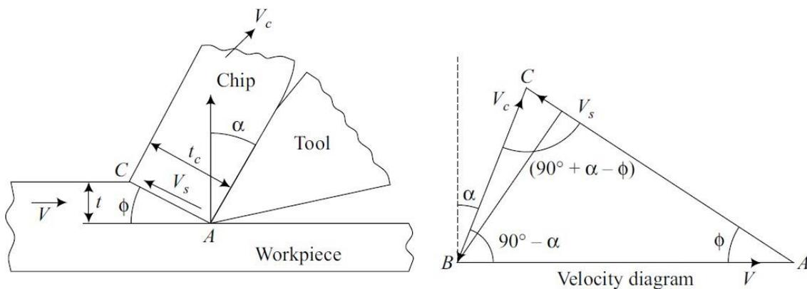
From velocity triangle  $BAC$ , using Lami's theorem,
