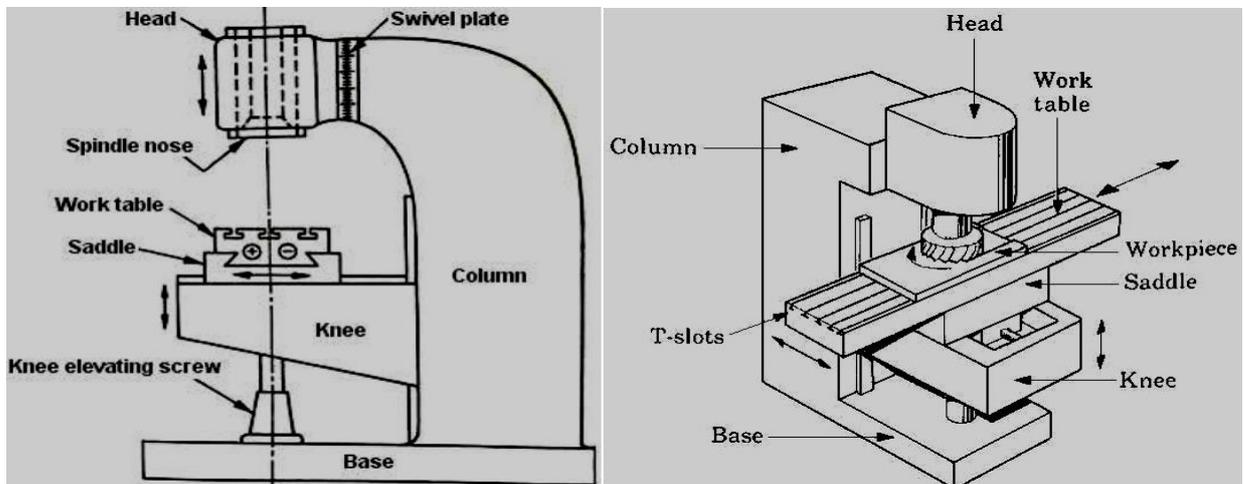
Fig. Vertical milling machine
