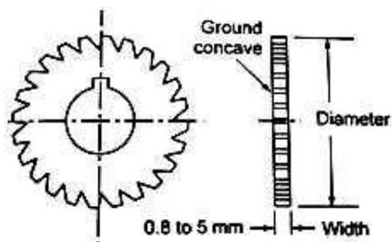
Fig. Slitting saw
