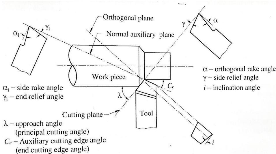
The angles are also measured in the plane (known as auxiliary reference plane) which is normal to the projection of the end cutting edge on the basic plane. These angles are end relief angle  $\gamma_1$  and back rake angle  $\alpha_1$  (also called auxiliary rake angle).
