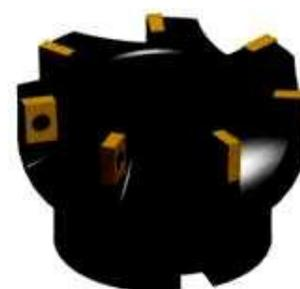
Fig. Face milling cutter
