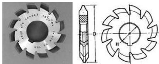
Fig. Involute gear milling cutter
