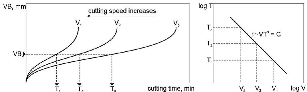
**Fig. Effect of cutting speed on wear land width and tool life for three cutting speeds. Natural log-log plot of cutting speed versus tool life.**
