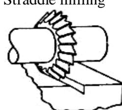
Fig. Form milling operations
